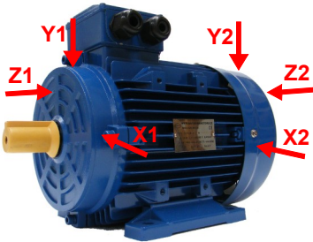
Figure 13: Measuring Points on Electric Motors
